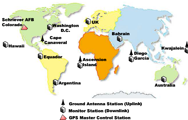
Fig. 2. Ground Station Global Positioning System
