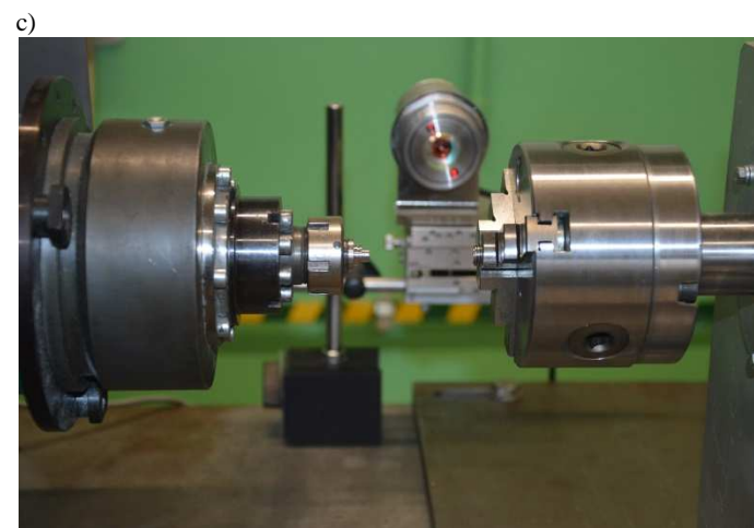
Fig. 3. Welding setups: a) laser welding, b) plasma welding, c) high speed rotational friction welding
