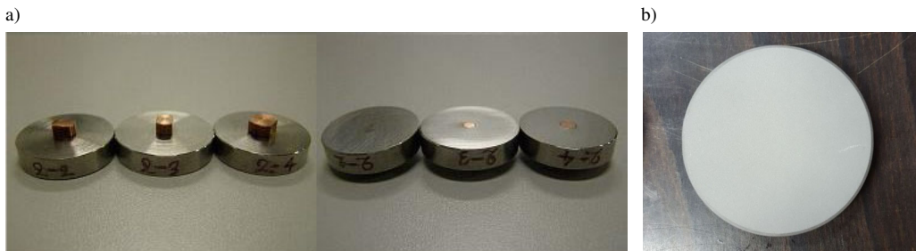
Fig. 2. Tested samples during the production of the adhesion defect (a), picture of one of the reference-coated samples (b), [18].
