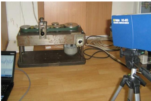
Fig. 2. The contactless measuring of vibration by the laser vibrometer
