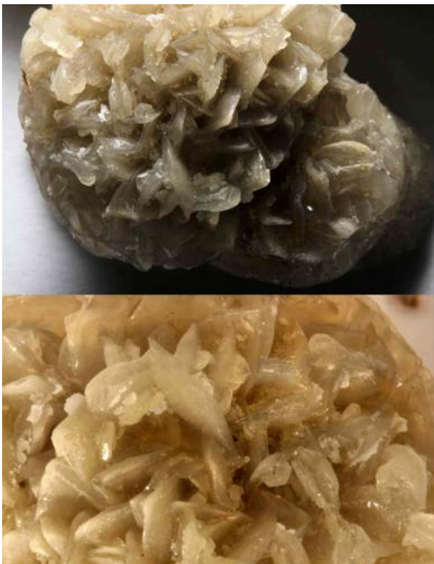
Fig. 13. – Gypsum crystals of the thornstone, graduation tower Bad Kösen. The width of the upper photo corresponds to approx. 3.0 cm and the width of the lower photo to approx. 1 cm.
