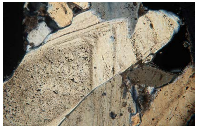
Fig. 15. – Microscopic close-up of gypsum crystals (crossed polarisers). The image diagonal corresponds to approx. 1 mm.
