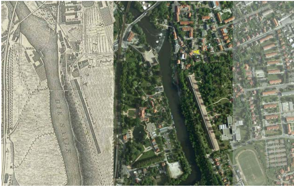
Fig. 5. – A section of a historical map (BUDDE 2007) and an overview of the current center of Bad Kösen. The flatrod constructions are positioned north of the graduation tower. They connect the waterwheel with the brine pumping equipment of the Borlach shaft (yellow arrow) and the graduation tower.
