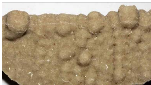
Fig. 10. – Part of a gypsum layer with an average thickness of 0.4 mm. The layer was formed on a timber profile at the passage of the graduation tower in Bad Kösen. The width of the photo corresponds to 11 cm.
