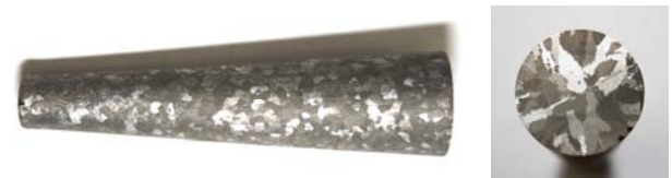
Fig. 9. Macrostructure of side surface and cross-section of test casting (1570°C, blue mould, blue filter)
