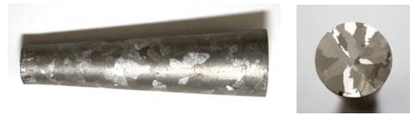
Fig. 6. Macrostructure of side surface and cross-section of test casting (1480°C, white mould, blue filter)
