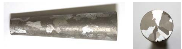
Fig. 8. Macrostructure of side surface and cross-section of test casting (1570°C, white mould, blue filter)
