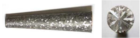
Fig. 7. Macrostructure of side surface and cross-section of test casting (1480°C, blue mould, blue filter)
