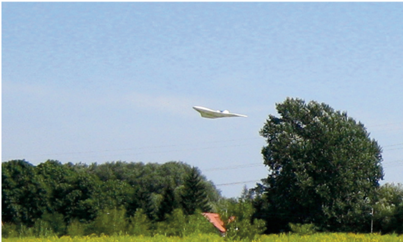
Fig. 10. MAV with foam shell structure in flight
