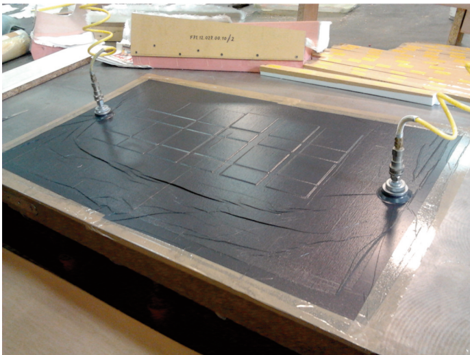
Fig. 7. Set of composite structure samples with integrated hinges
