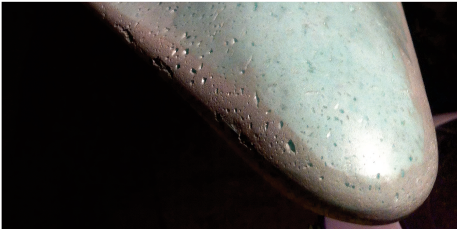
Fig. 14. Rough surface with holes of the two component foam structure
