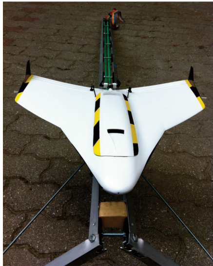
Fig. 1. Flight tested MAV with composite structure
