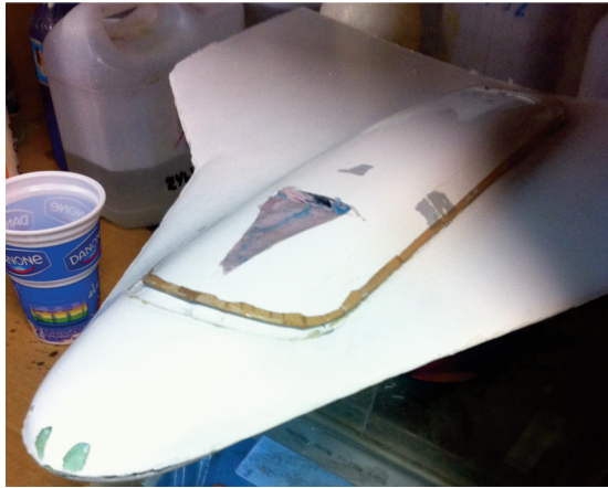
Fig. 6. The single ply composite structure with air bubble defects
