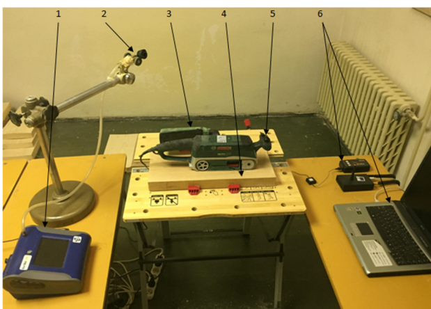
Fig. 1 Layout of experiment: 1 – aerosol monitor, 2 – IOM sampler, 3 – belt sander, 4 – spruce plank, 5 – pressure force sensor, 6 – pressure force monitoring system
