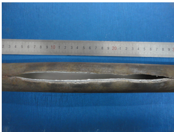
Figure 13. Picture of Specimen 4 with a big longitudinal opening
