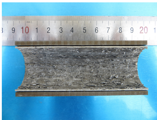
Figure 2. Ablation phenomenon in the surface of Al-Steel pipe by the old explosive welding method
