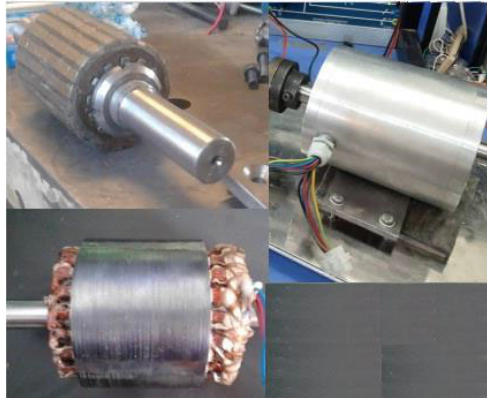
Fig. 7. Rotor core, stator core with windings and prototyped machine
