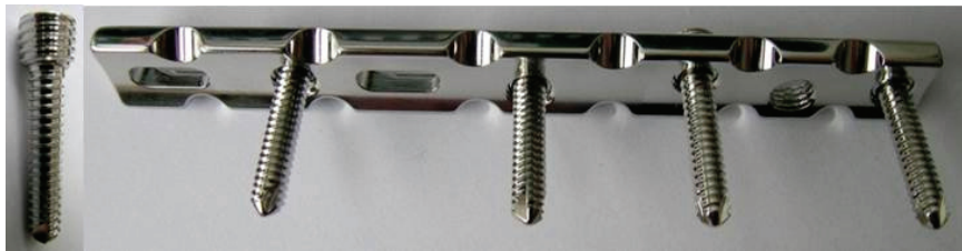
Fig. 1. Low contact compressive plate being analyzed
