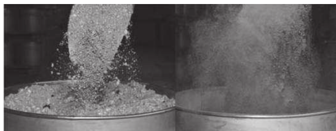
Fig. 1. Images showing aluminium powders, on the left – DEPUVAL aluminium; on the right – flaked powder [8]
