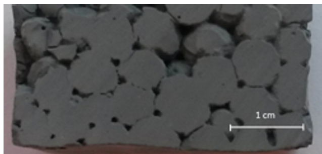
Fig. 2. Cross-section of a porous SiC preform
