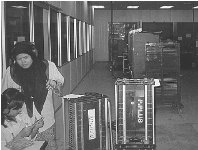
Figure 2. To minimise noise spreading to the manual component insertion area, noisy machines were confined to isolated areas. Operators were required to wear earplugs while entering those areas.
