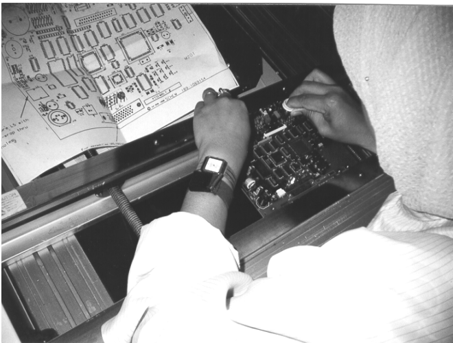
Figure 3. Finger work aids were used for pressing sharp top-edged and tight components.
