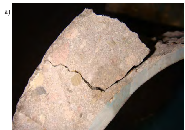
Fig. 9. Close-up of samples after the test: a) concrete pipe with liner and b) vitrified clay pipe with liner
