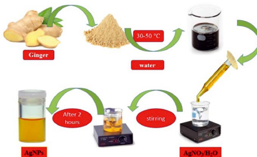
Figure 3. Schematic drawing of AgNPs synthesis (ginger extract is used in the green synthesis of silver nanoparticles as both a coating agent and a reducing agent; silver nitrate solution ( \text{AgNO}_3/\text{H}_2\text{O} ) and ginger extract (5 mL) was mixed with stirred continuously; UV-Vis spectroscopy or color change of solution represented the formation of silver nanoparticles 38 )
