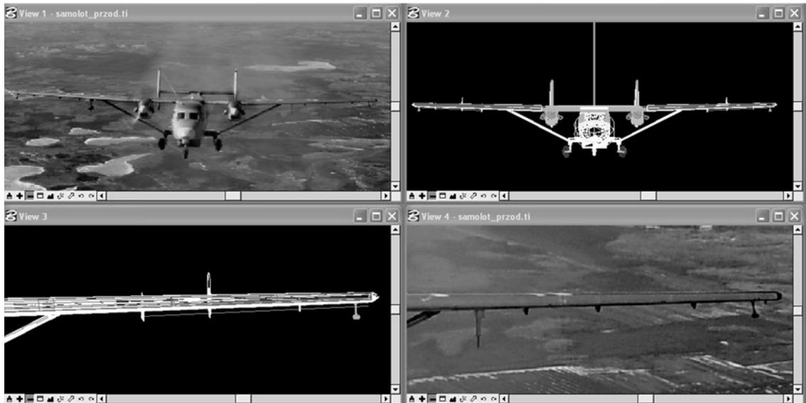
Fig. 6. The view of the program Image Analyst and MicroStation with CAD model and the image recorded during the flight
