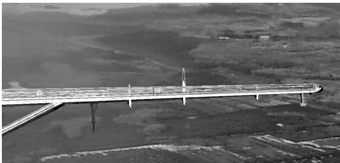
Fig. 8. Overlapping the digital image on CAD model
