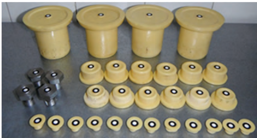
Fig. 4. Test adapters printed in 3D technology
