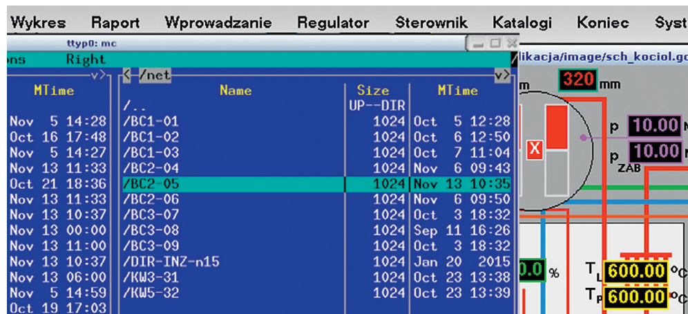
Fig. 5. QNX6-Qnet protocol – transparent access to operator station files in the local network
