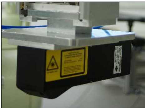
Fig. 9. Laser scanner module and its basic parameters [14]
