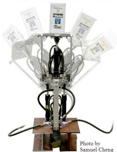
Fig. 1. Hydrobot – The Modular Electro-Hydraulic Robot Arm [3]
