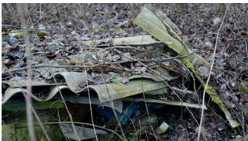
Fig.7. Asbestos-cement boards left next to fencing of the heap [M. Glica].
