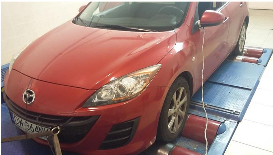
Fig. 1. Object of NVH tests mounted on the chassis dynamometer LPS3000
