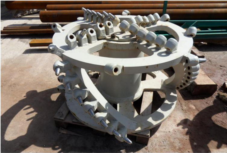
Fig. 3. Spatial cutting head used for salt beds mining in shaft SW-4
