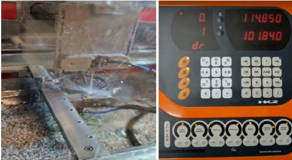
Figure 1. ZAP BP 800 wire electrical discharge machine (workstation and cutting area are shown)
