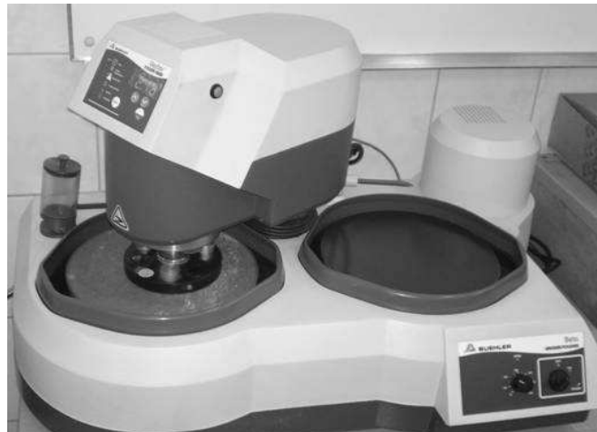
Fig. 2. The overall view of the Beta 2 dual platen grinder-polisher machine equipped with Vector power head and specimens holder
