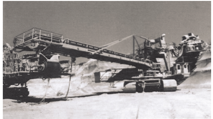
Fig. 1 Discharge boom of C700S excavator in the Kolubara open cast mine
