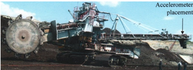
Fig. 17. Reconstructed BWE C700S discharge boom on the Kolubara open-cast mine
