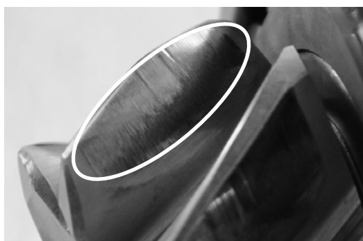
Fig. 1. Scuffed area on the tooth flank of a spiral bevel gear (in the white ellipse)
