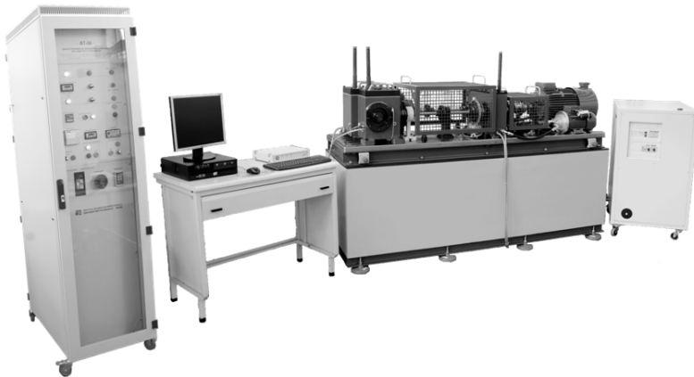
Fig. 2. Test spiral bevel gears (a), and T-30 Back-to-back bevel gear test rig (b)
