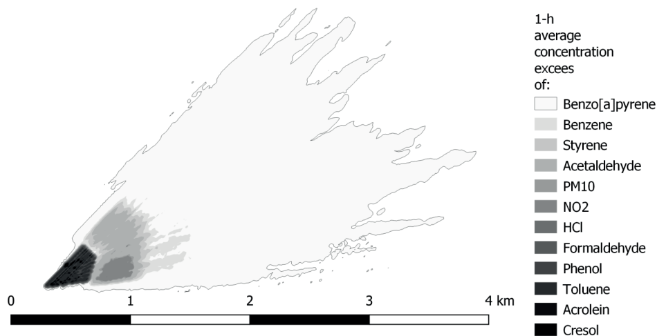
Fig. 2. Map of dispersion of substances with an impact range larger than 500 m emitted during a fire of 300 Mg municipal waste.
