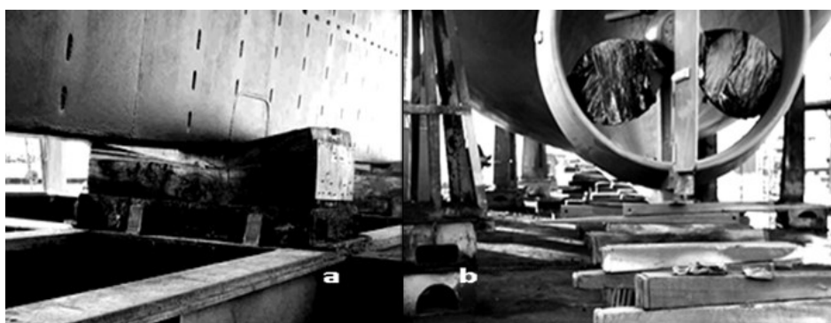
Fig. 4. Wooden keel blocks under vessels with reinforced keel.
