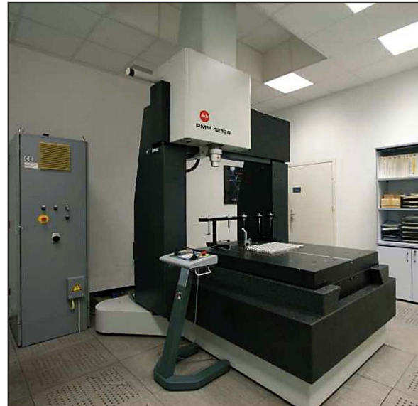
Fig. 1. Coordinate Measuring Machine PMM 12106 from Leitz
