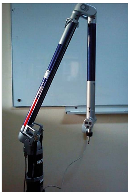
Fig. 2. Coordinate Measuring Arm Omega from Romera
