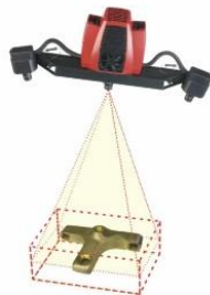
Fig. 3. Example of measuring strategy A: object smaller than the measuring volume of the scanner
