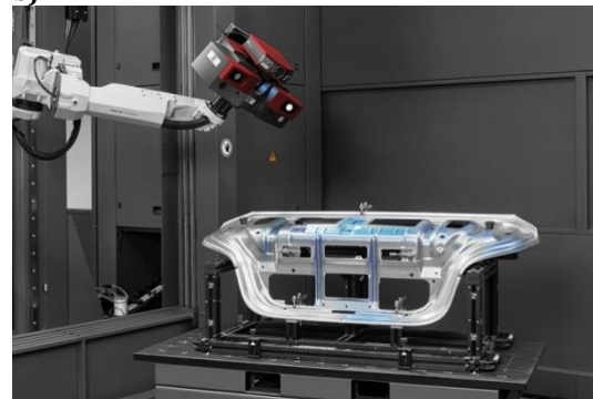
Fig. 1. Control and measurement resources: a) Zeiss PRO [15]-boom machine; b) automated measuring station with an optical scanner [16]
