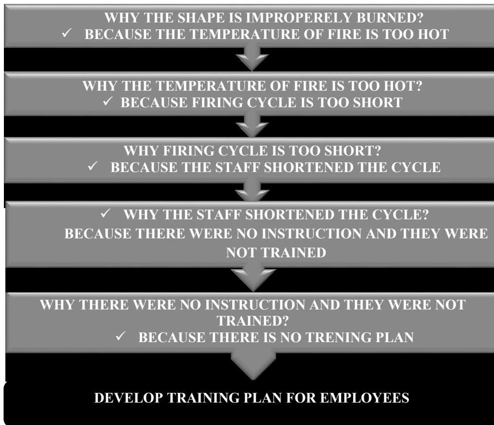
Fig. 5. 5 WHY analyze for incorrect type of wrongly burned shape Source: Author's own work.
