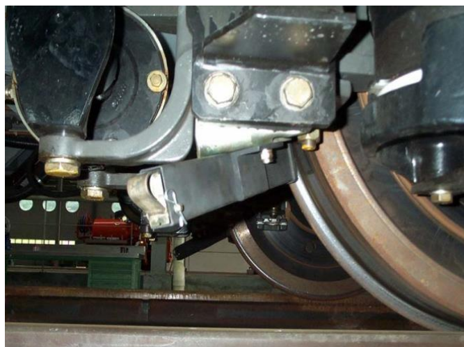
Fig. 5. Tram wheel flange lubrication device [13]
