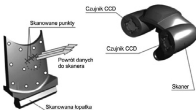
Rys. 1. Proces skanowania skanerem ZScanner 700 Fig. 1. Scanning process using ZScanner 700
