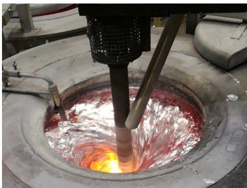
Fig. 1. Flux addition during rotary degassing
