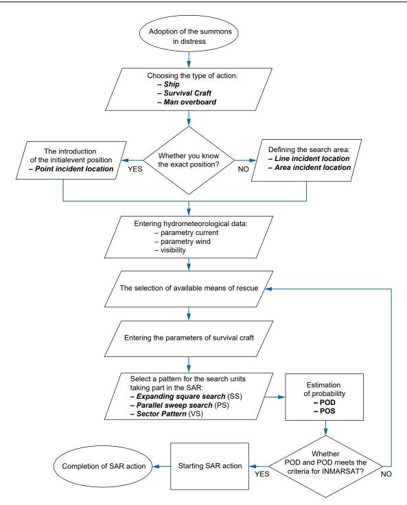
Figure 19. The block diagram of rescue action planning
