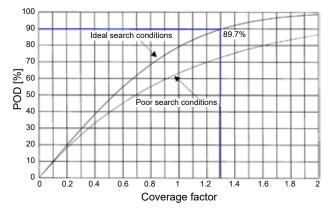
Figure 17. Average probabilities of detection (POD) over an area for visual searches using parallel sweeps (IMO, 2019a)
