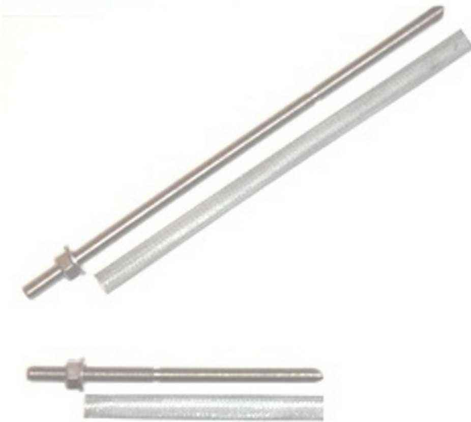
Figure 10. View of the COPY-ECO anchor system reinforcing the outer wall plates of large slab panel buildings: a) horizontal anchor M12 x 190 mm, b) oblique anchor M12 x 330 mm.
