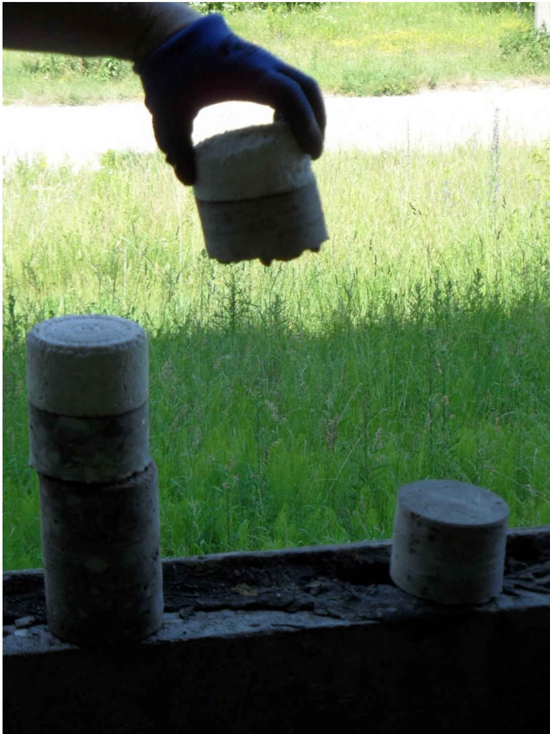
Figure 6. View of checking the cohesion of layers in the sample hole. [ref. own]
