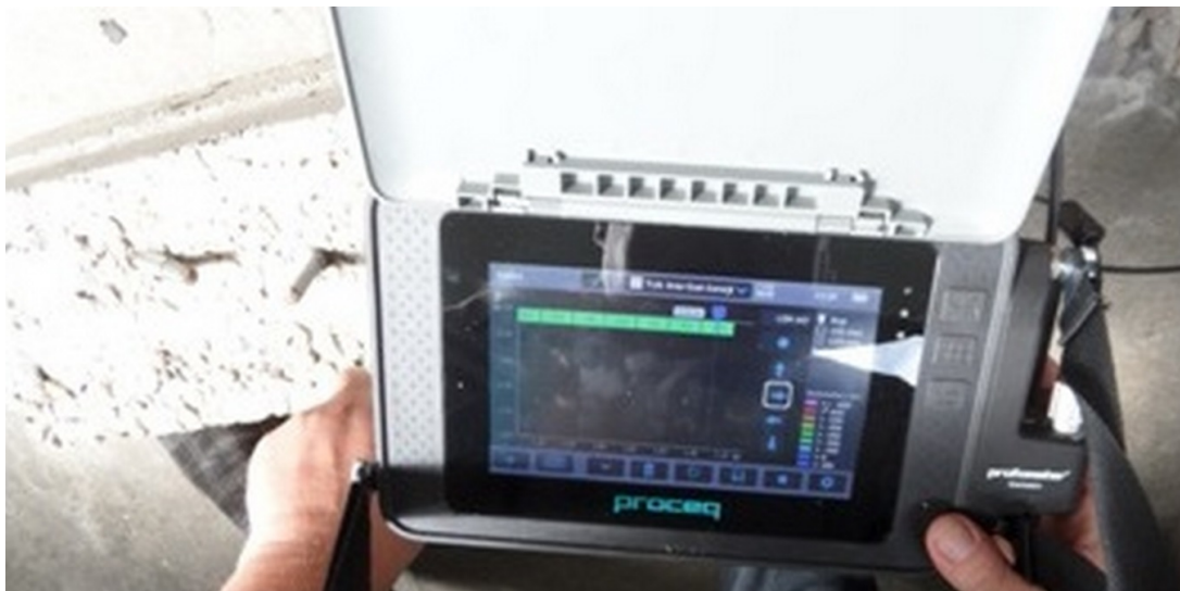
Figure 2. Preparation of the Profometer Corrosion for testing.
