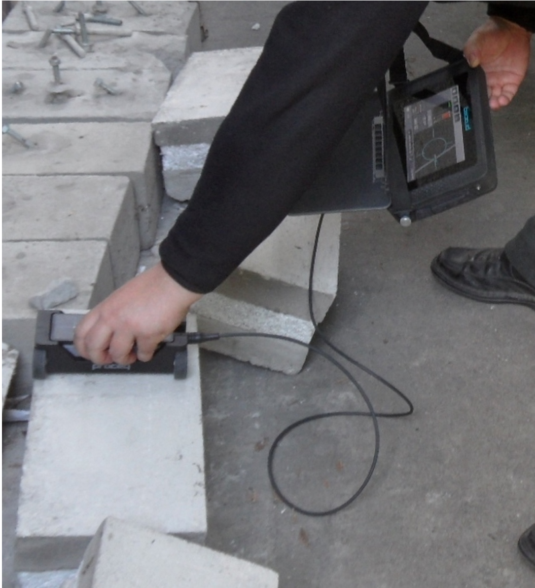
Figure 3. Preparation of the Profometer PM-650 for testing.
