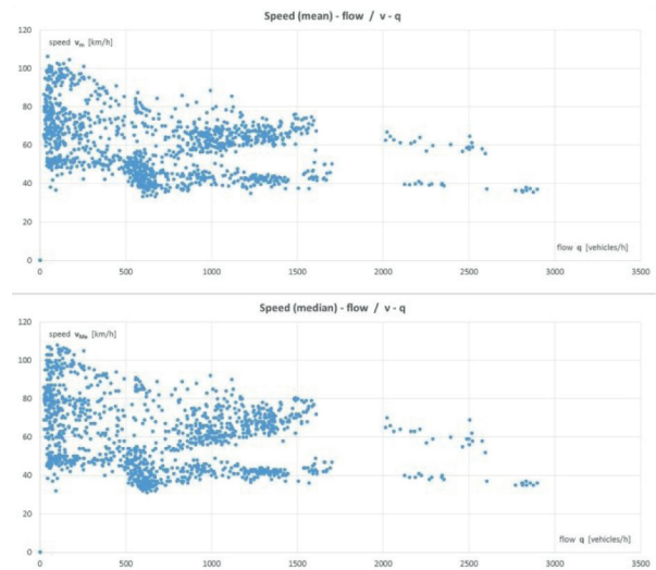
Fig. 9. Fundamental Diagrams for the second cameras location aggregated over 60 minutes. a) Fundamental diagram Mean Velocity vs Flow rate. b) Fundamental diagram Median Velocity vs Flow rate aggregated [own study]
