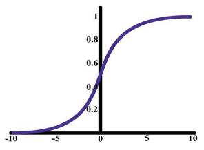
**Figure 3.** The nonlinear activation function that approximates the minimum and maximum values in asymptotes
