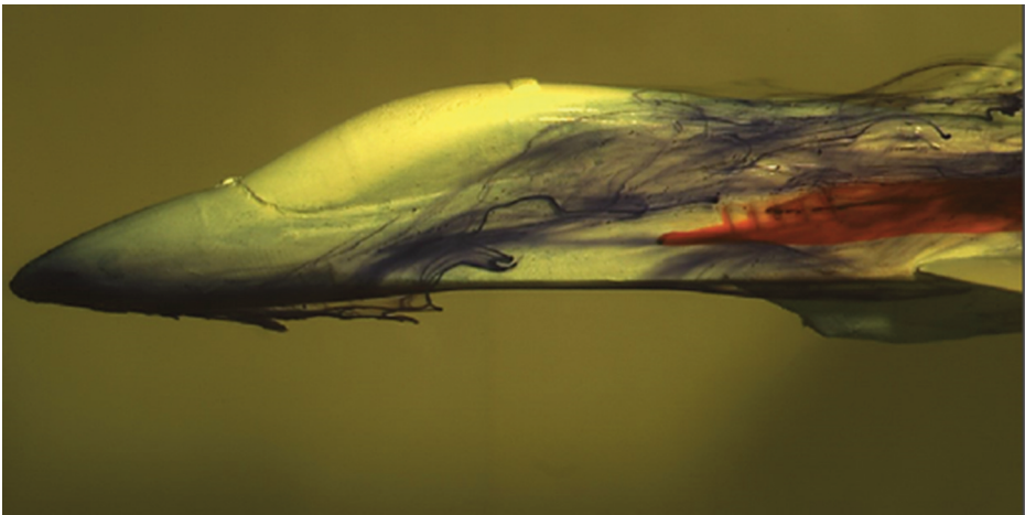
Fig. 3. Dye flow around an aircraft model [Szczeplaniak, 2015]
