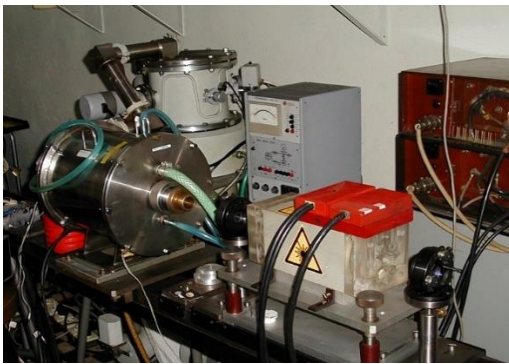
Fig. 6. Test stand for thermal diffusivity pulse testing of solids, designed by Professor J. Terpiłowski in 1975, and partly engineered at the National Centre for Nuclear Research in Świerk
