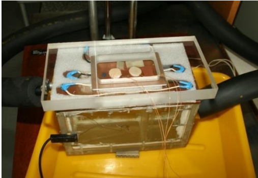
Fig. 9. Thermal diffusion test stand for the modified Angström method, by A. Panas (2005)
