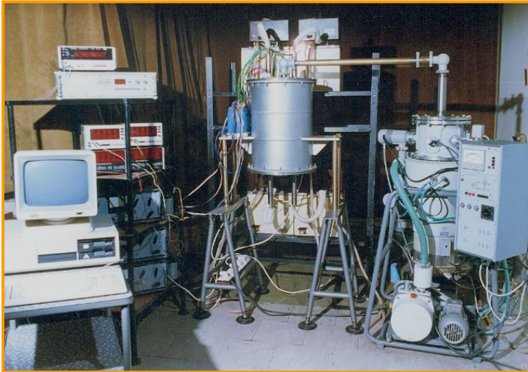
Fig. 4. Overview of the test stand for testing thermal conductivity of insulating materials from room temperature (RT) to 700°C, which was developed and built by Professor P. Koniorczyk at DAT in 1987 [6, 7]
