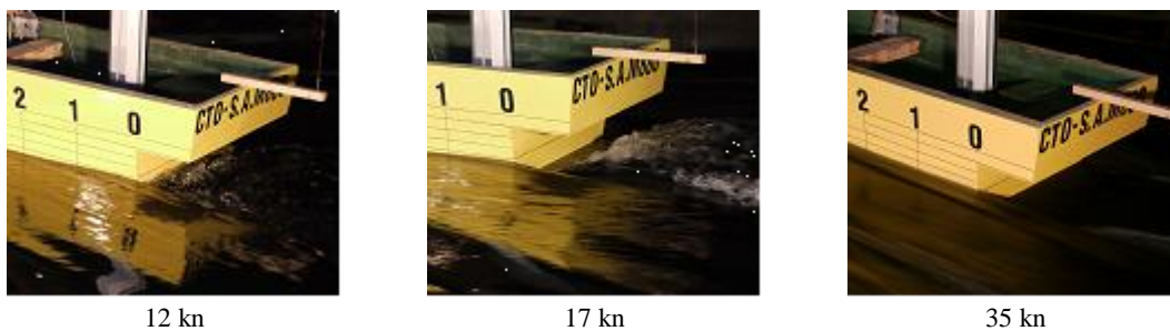
Fig. 4. Transom wave system evolution – high speed displacement vessel [CTO SA]
