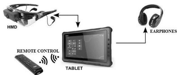
Fig. 1. Hardware configuration that allows using a tablet or a tablet with head mounted displays of an “Opticalsee-through HMD” type
