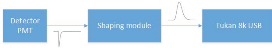
Fig. 1. The general scheme of the measurement system during the investigations.
