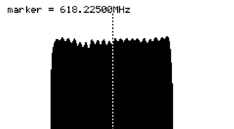
Rys. 6. Widmo cyfrowego kanału TV zmierzone wykonanym analizatorem Fig. 6. Spectrum of the digital TV channel measured by analyzer built by the author
