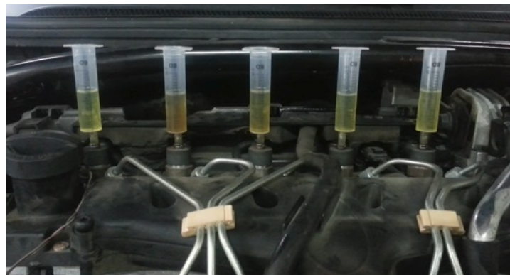
Fig. 5. Measurement of the volume of injector overflows [3]
