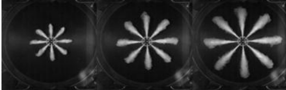
Fig. 6. Propagation of the fuel spray for an 8-hole injector [4]
