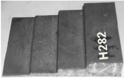
Fig. 4. Step g \times 35 \times 150 mm H282 alloy casting used in the conducted tests; g denotes the thickness of each „step”
