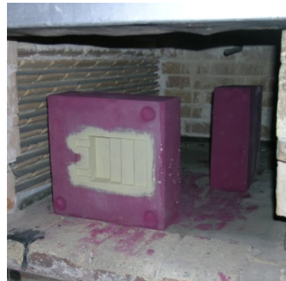
Fig. 2. A dry two-part mold for the technological “step” test
