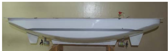
Fig. 7 Side view of the model with appendages
