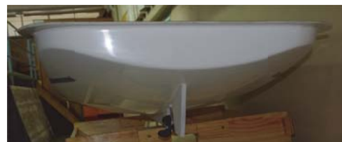
Fig. 9 Model without appendages during the test
