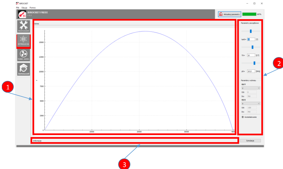
Fig. 6. The Simulation tab with its specific panes highlighted [3] (1 – Plot; 2 – Input pane for initial simulation parameters and plotting configuration; 3 – Auxiliary information drop-down pane)
