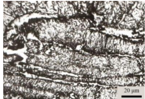
Fig. 6. Microstructure of GPC Ni-B+11Cr18MoWCu after heat treatment at T = 1110 °C, t = 2 min, 500 \times . GPC, galvanic plasma coating
